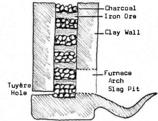
was reached the melted slag trickled out from the opening at the base of the shaft. The iron, a sponge-like mass, was left in the shaft. This had to be removed and reheated in an open bowl furnace and then hammered on an anvil.
