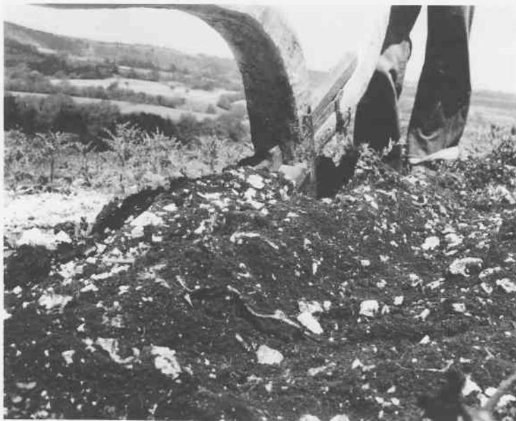
Plate 8. The bite of the foreshare and lift of the undershare.
