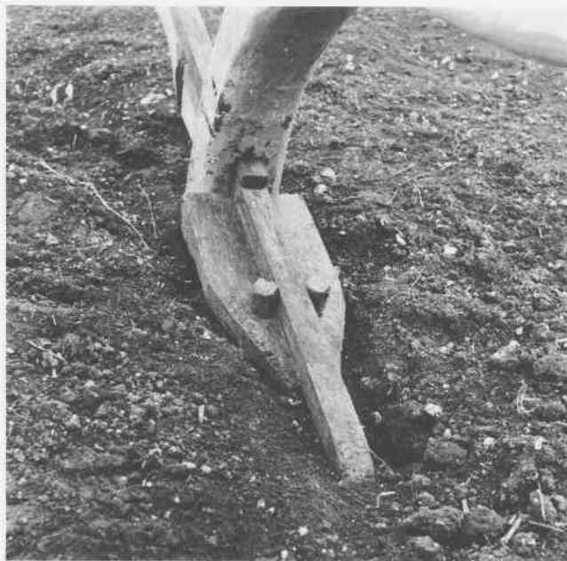
Plate 4. Detail of the foreshare and main or under share and fore wedge.
