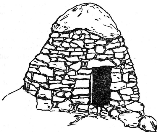
Fig. 1. A typical cleit for storing fuel or hay. Many date to the nineteenth century AD
